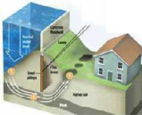
Piping and Uplift
